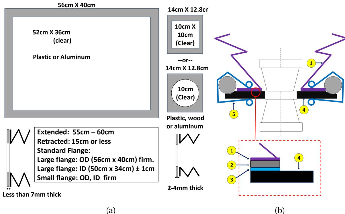
Figure 23: Bellows. (a) Bellows and flange information. (b) The bellows (1) is attached to the flange (2) which is attached to the lens-board (4) by steel clips (5). A layer of felt (3) is placed between the flange and the lens-board.
