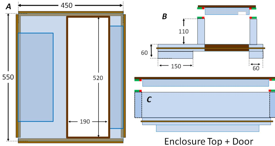
Figure 20: The top wall of the enclosure includes a box that provides a moving space for the vertical stage as well as access to the stages and sensor from the top through the door shown on the right. The green and red bars are a felt and magnet/metal pair respectively used to seal the door.
