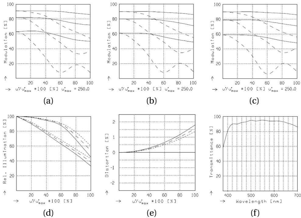
Figure 13: MTF of the Schneider 800/12 @ f22 and focal distance (OO') at  $\infty$  (a), 17.3m (b) and 9.5m (c). Spatial frequency is 5,10,20 lp/mm, solid lines are for radial orientation and dashed lines for tangential. (d),(e),(f) show the relative illumination, distortion and transmission of the lens. Note that our camera operates at 0.6 (vertical) 0.9 (horizontal) of the image circle size. Source: manufacturer web-site. Unaltered, faithful to original.
