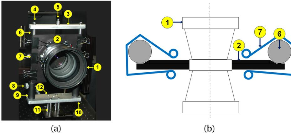
Figure 8: The lens holder. **(a)** 1: Lens, 2: Lens board, 3: Top bar, 4: M6 screw, 5: Auxiliary camera holder, 6: Steel post (12mm), 7: Steel clip, 8: Lock screw, 9: Post holder, 10: Base bar, 11: Steel post (8mm), 12: M4 screws. **(b)** The lens board is held by pressing the steel posts against grooves in the lens-board by steel clips. (The post holders support the lens board at the bottom). (image not to scale)
