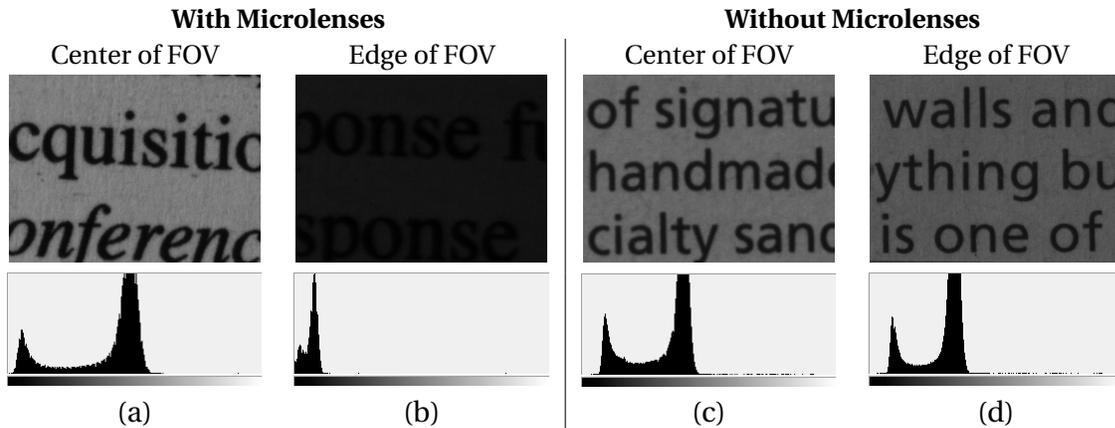
Figure 3: Microlenses are harmful for large format imaging. (a) and (b) are images (with their histogram shown below) taken by a sensor with microlens at the center and the edge of the field of view, whereas (c) and (d) are images taken by a sensor without microlenses. We can see that the image taken with microlenses is severely degraded at the edge of the FOV because sensors with microlenses are not designed to work with large format lenses.
