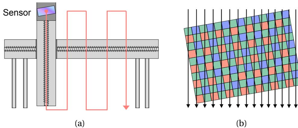
Figure 10: Image plane stage scanning. (a) the ZigZag motion minimizes the moving mass. (b) Rotating the sensor slightly about the optical axis (optional) allows scanning though all color channels.
