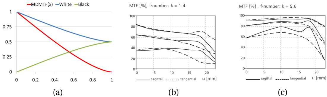
Figure 1: (a) Monochromatic diffraction limited MDMTF for a circular aperture X:normalized frequency, Y:Transmittance. (b),(c) MTF of the Carl Zeiss Planar T\* 1.4/50 standard lens for f-number 1.4 and 5.6 respectively Source: manufacturer web-site . Unaltered, faithful to original (b,c).
