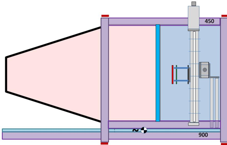
Figure 24: Optical window (blue) reduces the volume to be cooled and can significantly increase the cooling efficiency. **Not yet implemented**
