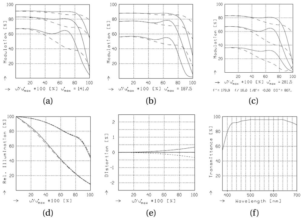
Figure 14: MTF of the Schneider macro 180/5.6 @ f15 and magnification factor (1/B') -2 (a), -1 (b), -0.5 (c). Spatial frequency is 5,10,20 lp/mm, solid lines are for radial orientation and dashed line for tangential. (d),(e),(f) show the relative illumination, distortion and transmission of the lens. Source: manufacturer web-site. Unaltered, faithful to original.
