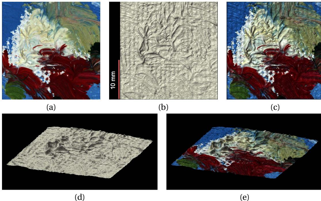
Figure 30: Controlled illumination for photometric stereo. **(a)** A flat color image of small patch of oil painting **(b)** 3D Texture recovered by photometric stereo. **(c)** Texture mapping. **(d,e)** A different view of (b,c).
