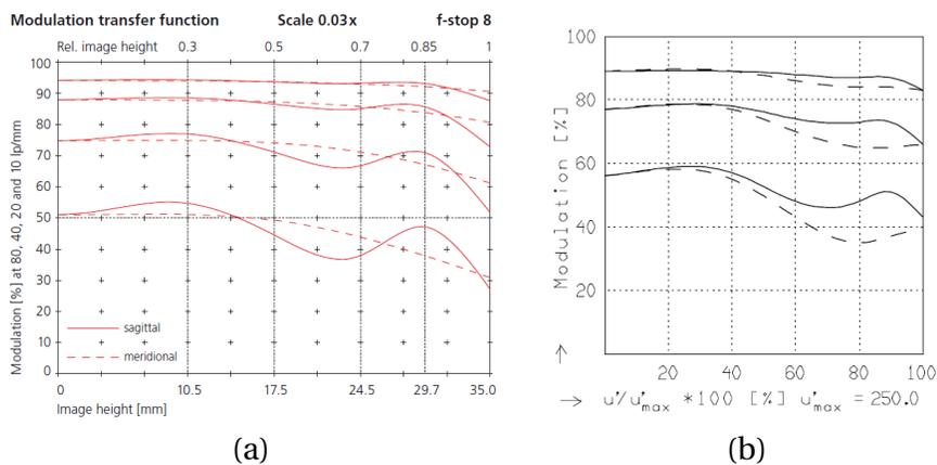
Figure 2: Modulation transfer function for the Rodenstock's HR Digaron-S 5.6/60 (a), and the Schneider Optics' APO SYMMAR 8.4/480 (b). The graphs show the MTF for spatial resolution of 10 20 40 80 lp/mm for the Rodenstock, and 5, 10, 20 for the Schneider's. Source: manufacturers web-site . Unaltered, faithful to original.
