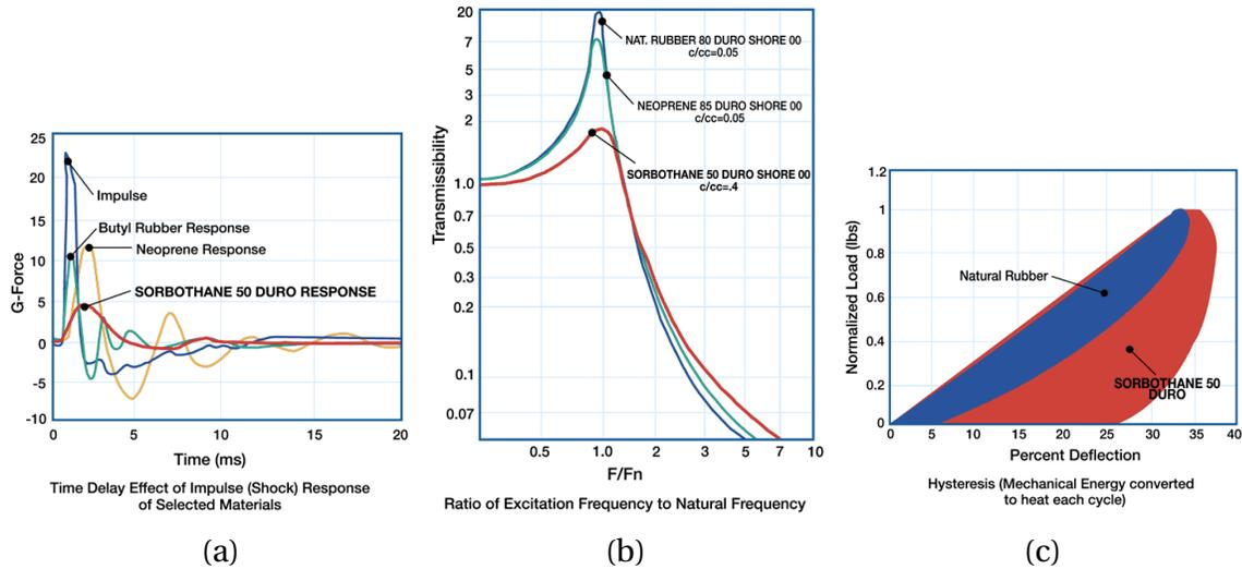
Figure 26: Sorbothane properties. **(a)** Response to shock **(b)** Vibration isolation **(c)** Energy dispersion.
