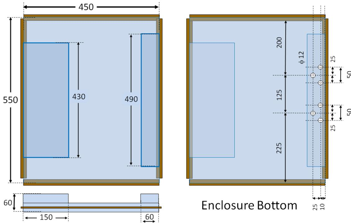
Figure 19: The enclosure bottom, or floor, is made similarly to the sides. The 6 holes in the right figure are for the steel posts that hold the horizontal translation stage.
