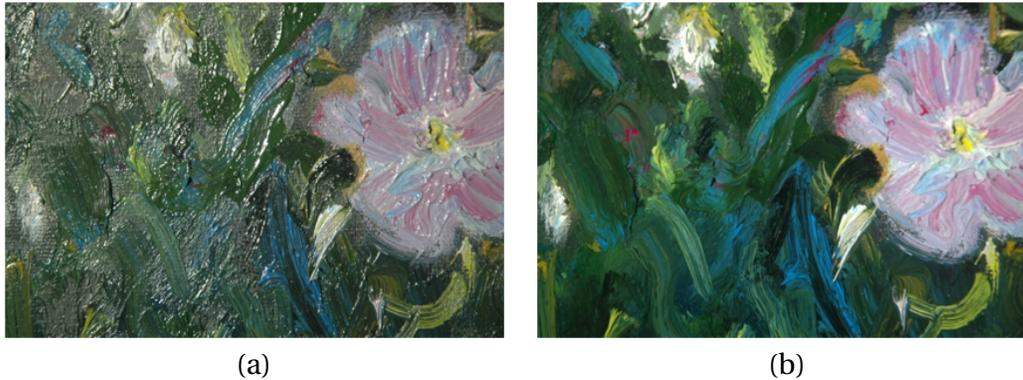
Figure 29: Cross polarization. **(a)** Aligned filter **(b)** Crossed filter. Highlights are highly polarized whereas the diffused reflection (of non metallic objects) is largely depolarized, this enables good suppression of highlights.
