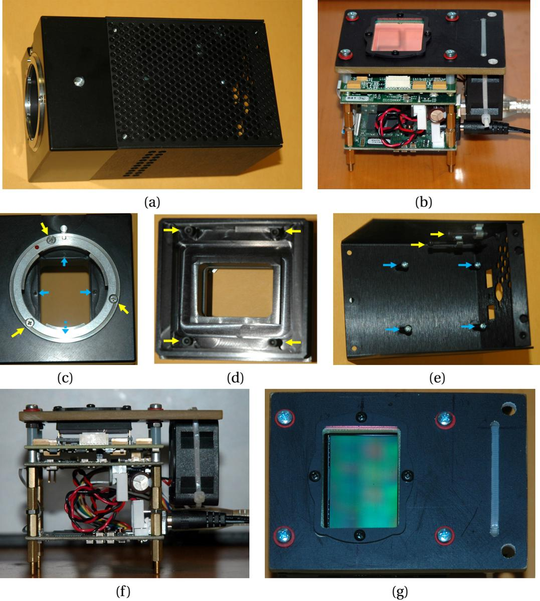
Figure 16: **(a)** Original camera enclosure. **(b)** Modified setup overview. **(c,d,e)** Open enclosure, arrows show screws locations. **(f,g)** Modified setup side and top view. Note images show temporary posts (20,21 in previous figure).
