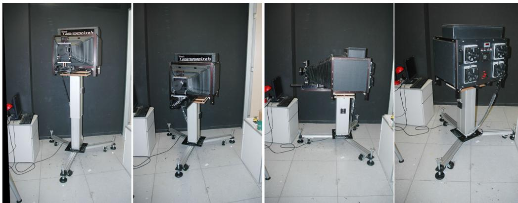
Figure 27: Camera pier and caddy: The camera is mounted on a telescope pier that allows for adjusting the height of the camera. A caddy allows the camera to move on wheels and firmly located using legs (that lift the wheels slightly off the ground).
