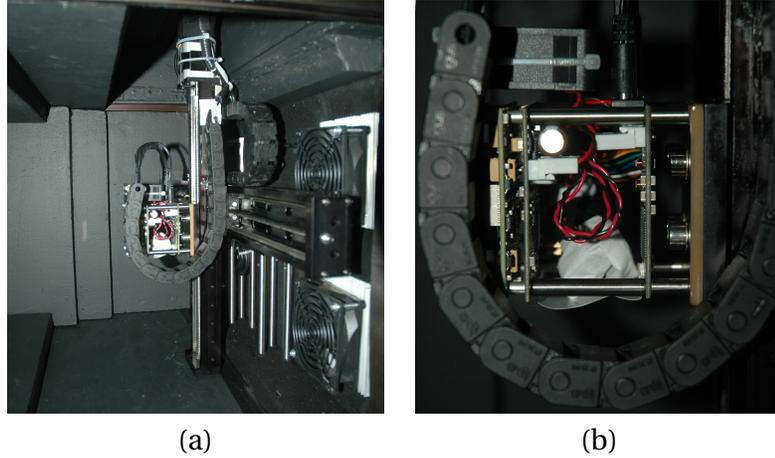
Figure 17: **(a)** Power and USB wires to the camera are guided via wire guides. **(a)** Closeup at the sensor. The wire guide is attached to the edge of the top plate. Note: Final steel posts (20,21) and connection to the translation stage (23) are shown in this image.
