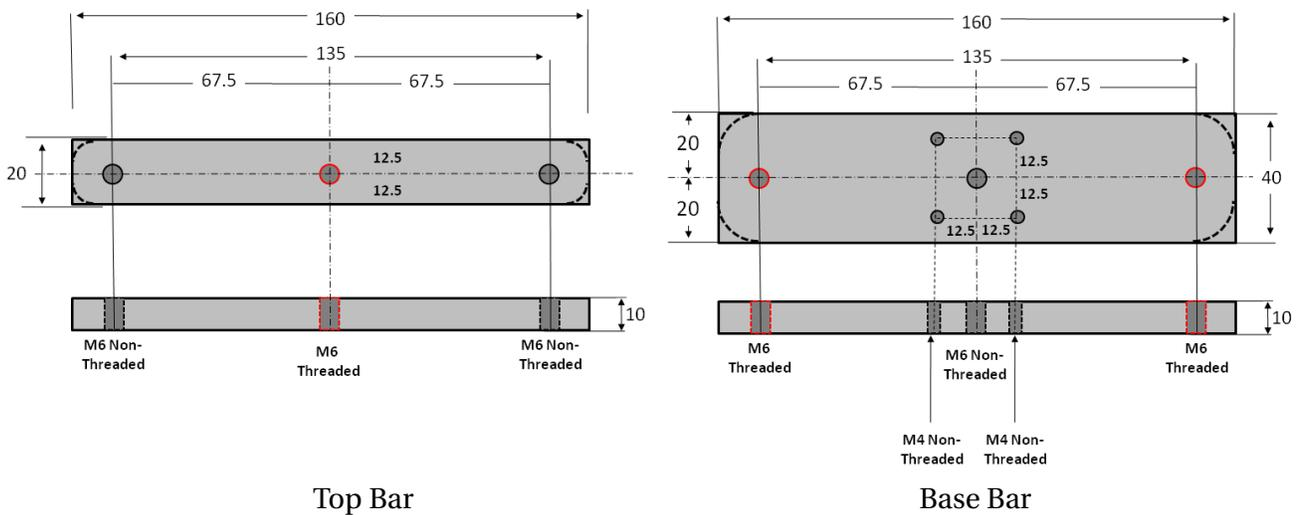
Figure 9: Lens holder custom made aluminium bars. All measures in mm.
