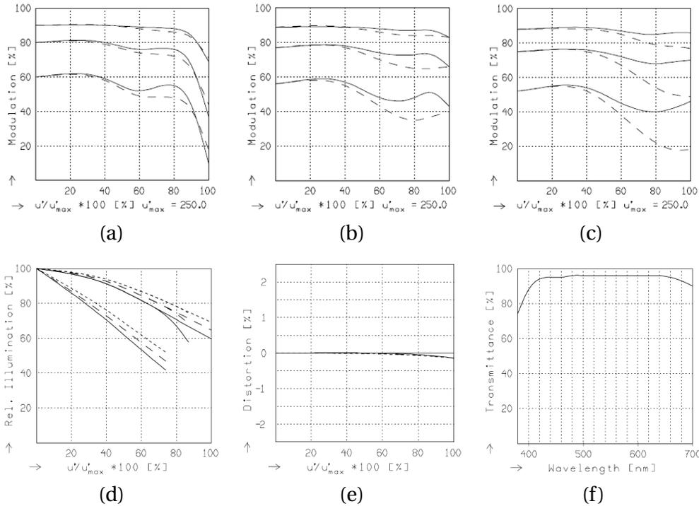
Figure 11: MTF of the Schneider 480/8.4 @ f22 and focal distance (OO') at  $\infty$  (a), 5.6m (b) and 3.3m (c). Spatial frequency is 5,10,20 lp/mm, solid lines are for radial orientation and dashed lines for tangential. (d),(e),(f) show the relative illumination, distortion and transmission of the lens. Note that our camera operates at 0.6 (vertical) 0.9 (horizontal) of the image circle size. Source: manufacturer web-site. Unaltered, faithful to original.
