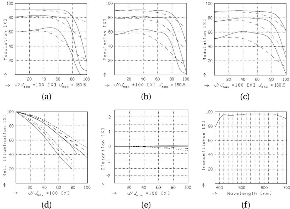
Figure 12: MTF of the Schneider 210/5.6 @ f22 and focal distance ( $OO'$ ) at  $\infty$  (a), 2.5m (b) and 1.5m (c). Spatial frequency is 5,10,20 lp/mm, solid lines are for radial orientation and dashed lines for tangential. (d),(e),(f) show the relative illumination, distortion and transmission of the lens. Note that our camera operates at 0.6 (vertical) 0.9 (horizontal) of the image circle size. Source: manufacturer web-site. Unaltered, faithful to original.
