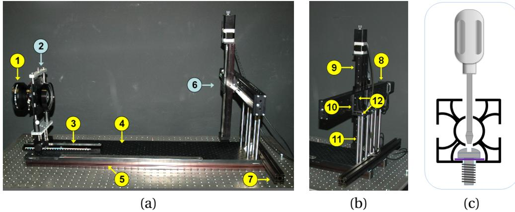
Figure 7: The skeleton of the camera. **(a),(b)** (1:Lens), 2:lens Holder, 3:Focusing Stage (manual) 4:Breadboard, 5:Supporting rail, 6:Image plane stages, 7:First enclosure rail, 8:Horizontal stage 9:Vertical stage, 10:Angle Bracket, 11:Steel post (12mm), 12:M6 screws. **(c)** Tip - to attach a rail to the breadboard, slide the screw through the rail, and drill a hole for the screwdriver (Philips type preferred).
